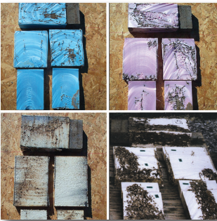
Termite-Damaged Untreated Foams
